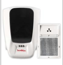
Addressable smoke detection system, linear optical reflection type. Optical attenuation detection technology of the reflected infrared beam. The TFMIID-120 detector is equipped with an OAS (Optical Alignment System) automatic servo-assisted alignment system, covered by an international patent. System composed of two devices, the detection and control panel and the reflection and telemetry unit.
