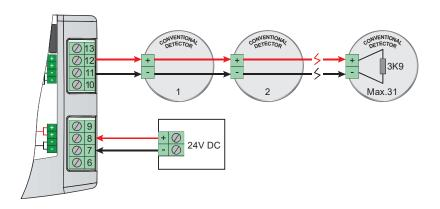
**NB** The connection line of conventional detectors must be terminated with a 3K9 ohm resistance, connected in parallel to the power supply of the last detector.
