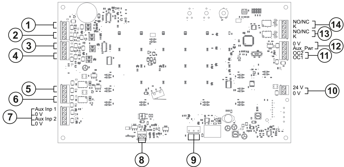
Figure 11: 2 Zone and 4 Zone main system board termination details
