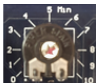
Figure 10: Normal potentiometer denoting time in minutes for setting the delay
