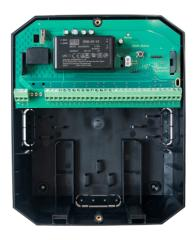
MultiTransmitter comes in a protective container with a dedicated space for a rechargeable battery.
